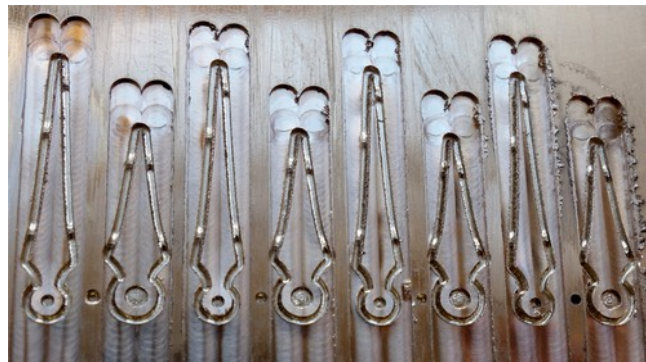
Prototyping of new GoS bronze hands with bevels yet to be handpolished
