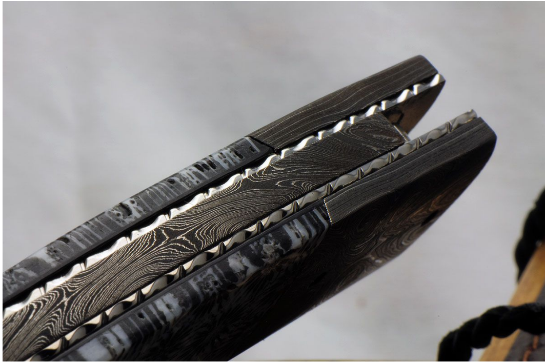
File work on Titanium liner in a Johan Gustafsson folder knife
